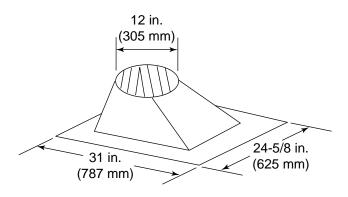
**RF371 Roof Flashing**
